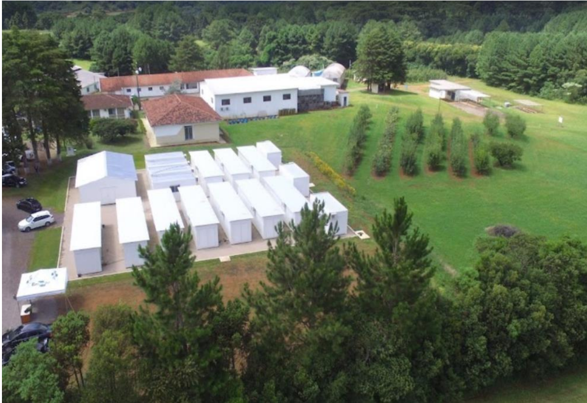
Figure 7. MOSCASUL Biological Control and Integrated Fruit Fly Management Center from EMBRAPA Grape & Wine at Vacaria, Rio Grande do Sul, Brazil. This fruit fly facility adopted a modular system with containerized laboratory modules for each stage of the insect.
